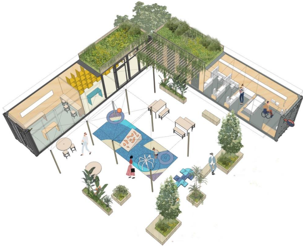
Design for toy library, toilets and public space, using shipping containers. © PiM.Studio Architects.
