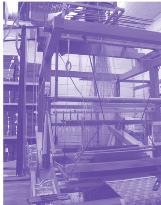
A jacquard mechanism attached to a treadle loom, Tatsumura Kôhō's workshop, Kyoto, October 2012.
