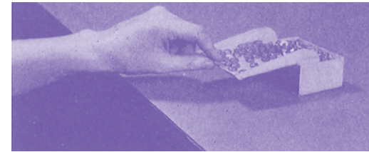
Example of bin meant to facilitate "select" and "grasp" of parts. Credit: Ralph M. Barnes. 1937, image. From: Motion and Time Study . New York: John Wiley & Sons, 1937.
