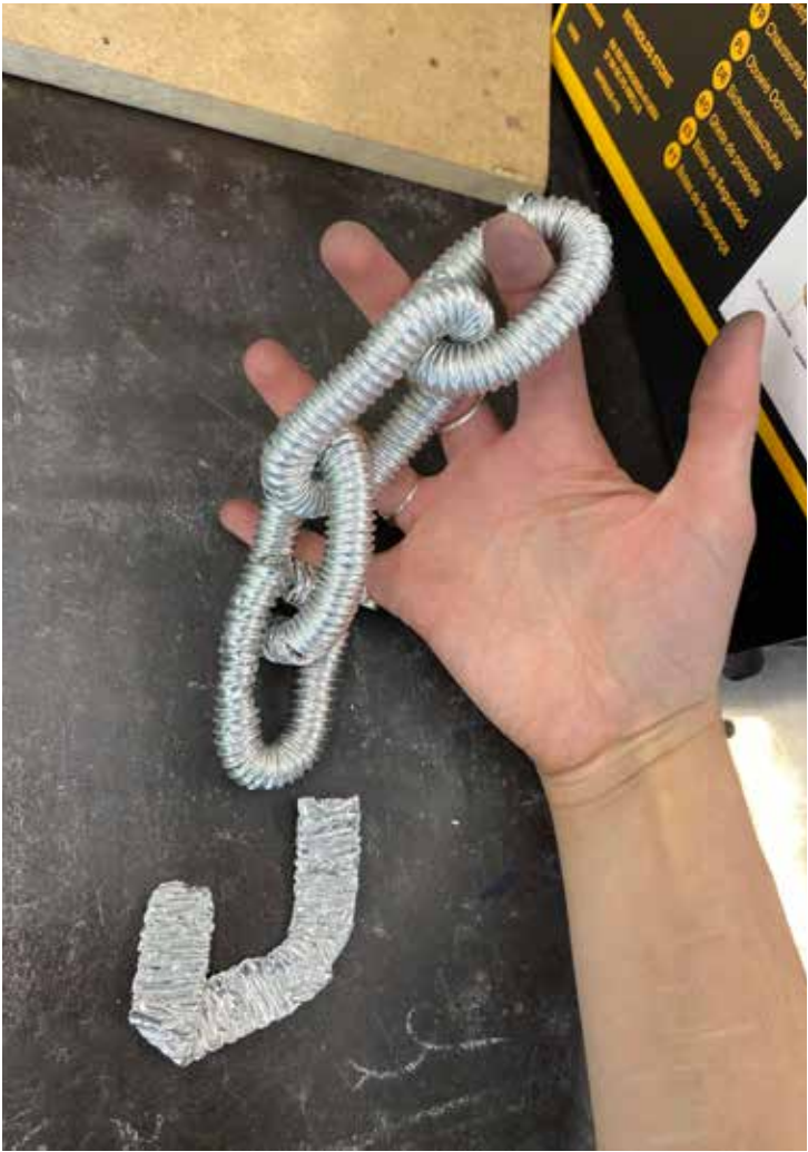
FIGURE 9 Making a chain link out of an old aluminium air vent.
