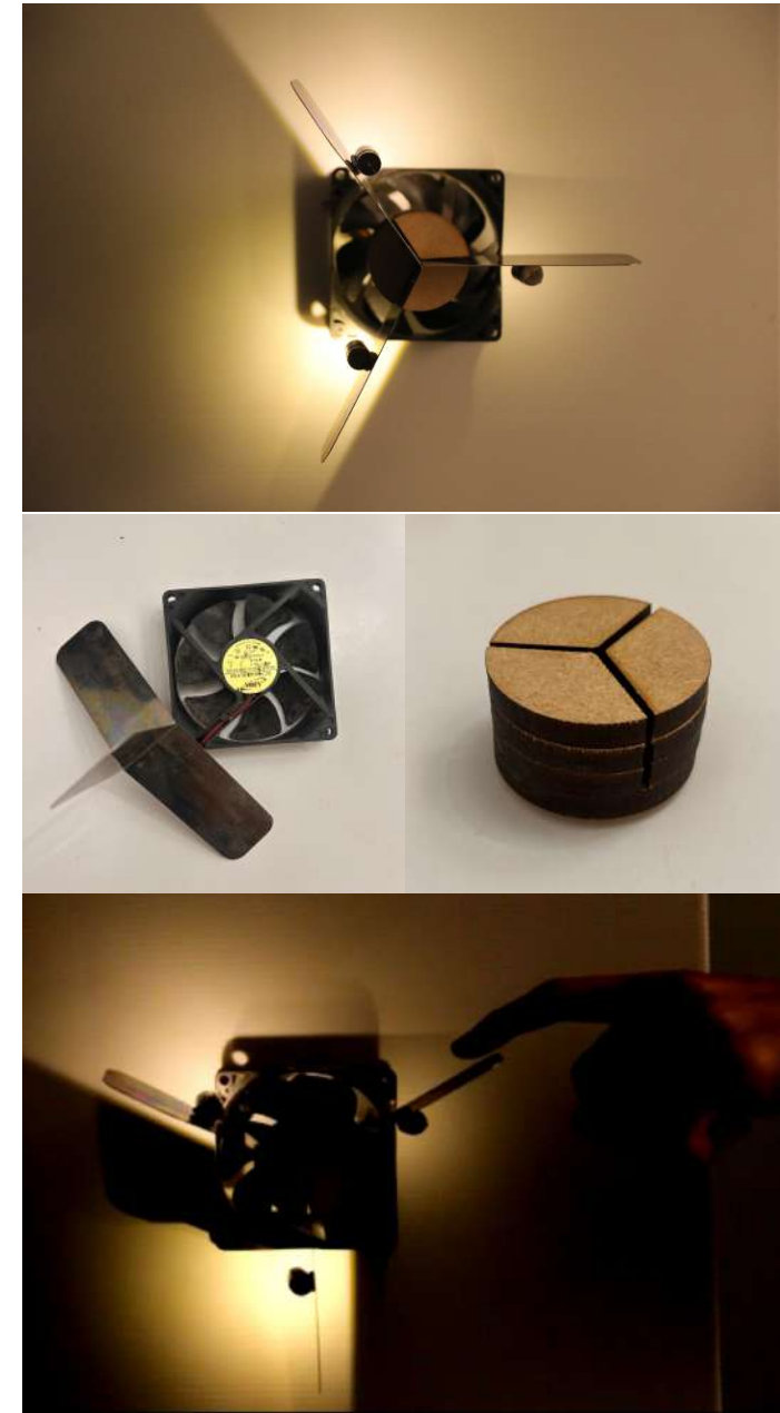
Playful wall mounted light made using a discarded computer fan and a part from a kitchen appliance. Mounted with glue and laser cut mdf. Click here for the video.
