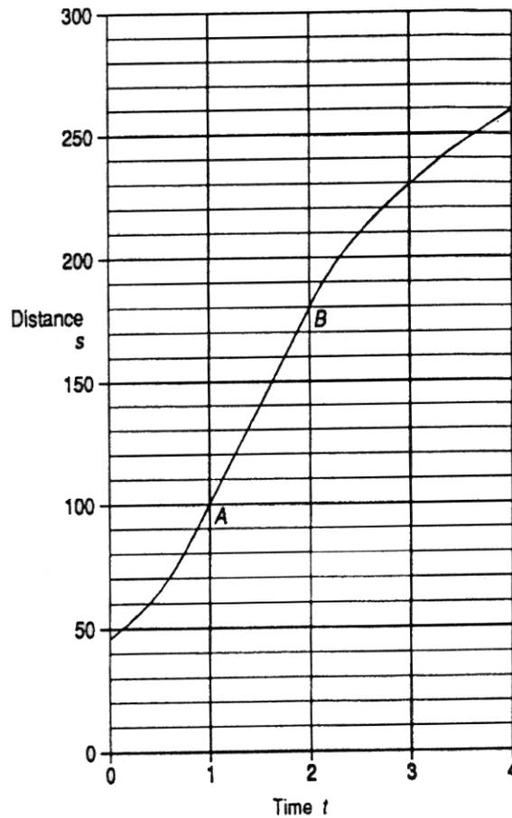
In this graph of distance (miles) against time (hours), the speed is varying all the time except in the region A – B. In that region the graph is a straight line, and the gradient is 80 (the distance goes from 100 - 180 in the second hour), so the speed is 80mph.
