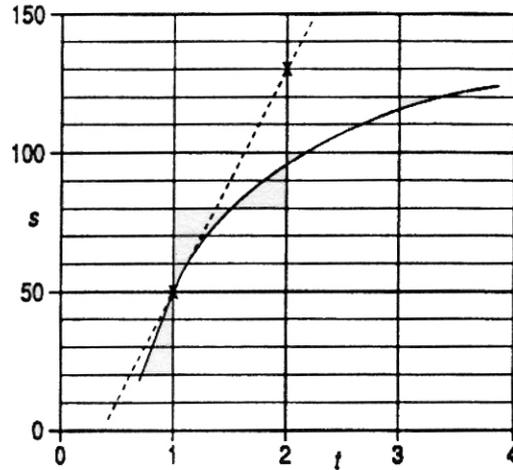
And now it can't be detected as a straight line region at all. But the gradient at A is still the same, and represents a speed of 80mph – that is what the speedometer would say at that moment. The dashed line is a tangent to the curve – that is a line which touches the curve at a point.
