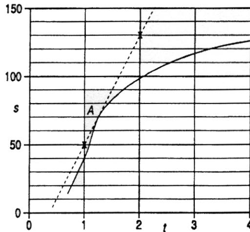
So the gradient of a curve at a point is the gradient of the straight line which touches the curve at that point.
