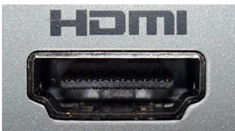
A HDMI input on a projector
