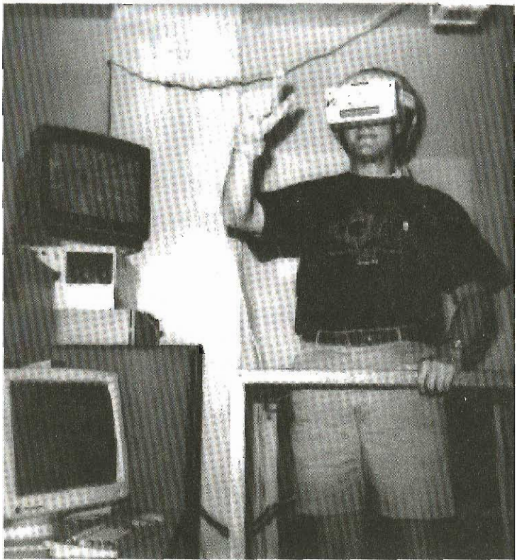
Figure I.1 A virtual reality head-mounted display. Courtesy of Professor Larry Hodges, GVU Center, Georgia Institute of Technology.
