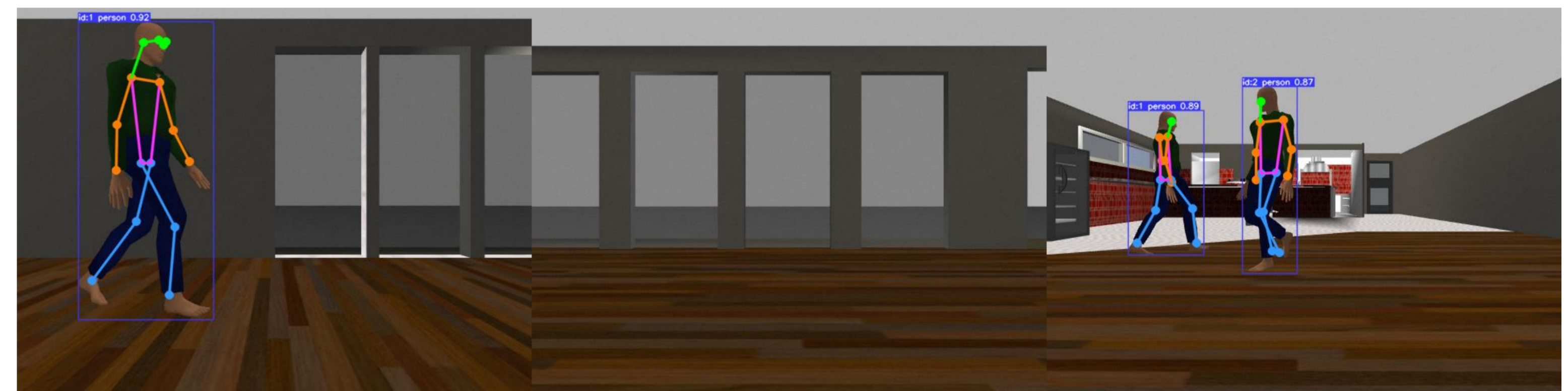
Figure 3: Fused image obtained from multiple cameras (front, right and left cameras)
