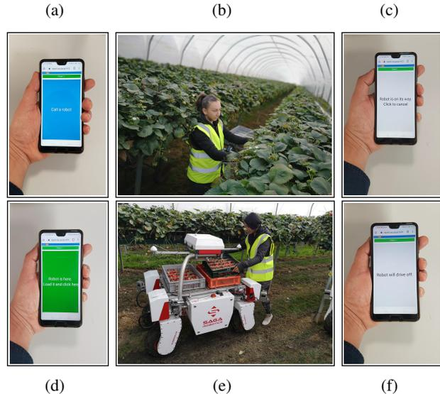
Fig. 1: A setup for an autonomous fleet of robots to support fruit pickers. Call-A-Robot (CAR) user interface: (a) ready to call a robot, (c) robot on the way to picker, (d) robot arrived at picker’s location and ready to be loaded, (f) robot sent to in-field storage with picked yield. A human picker picking strawberries (b) and loading full trays on a robot (e).
