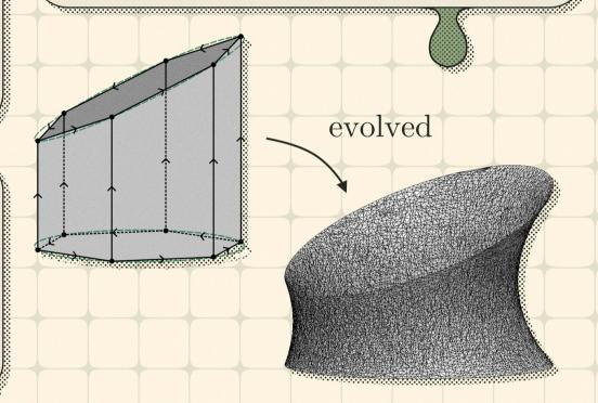
Using Surface Evolver, we were able to construct a model liquid bridge between surfaces at an arbitrary angle (measured in radians) to one another. Using Surface Evolver, we were then able to calculate the Gaussian curvature of these liquid bridge shapes and see how it varies as the angle between the surfaces changes.
