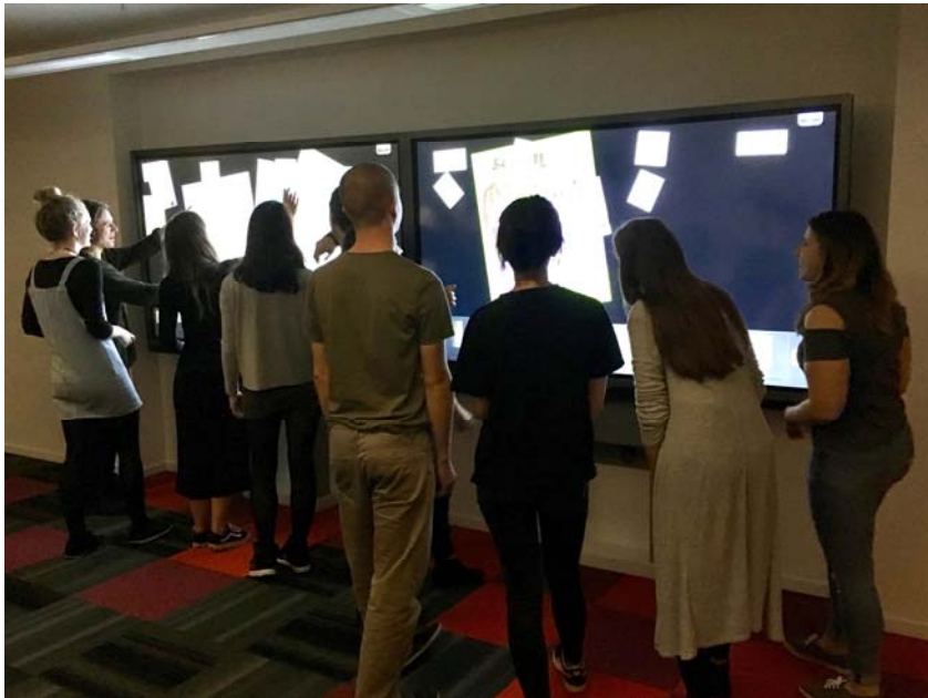
Figure 4: Each of the large touchscreens had sixteen active touchpoints facilitating effective group working.
