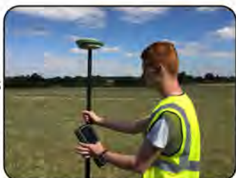
Fig 1. Use of a CS20 GPS to log points to an accuracy of 0.014M
