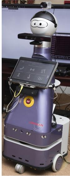
**Fig. 1.** RGB-D and thermal sensors mounted on top of a robot.
