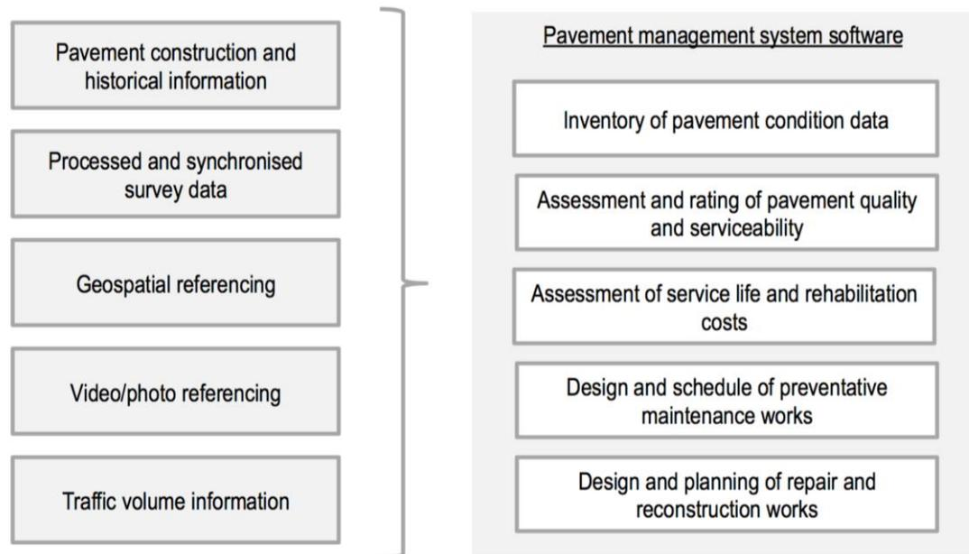
Figure 3. Pavement management system software inputs
