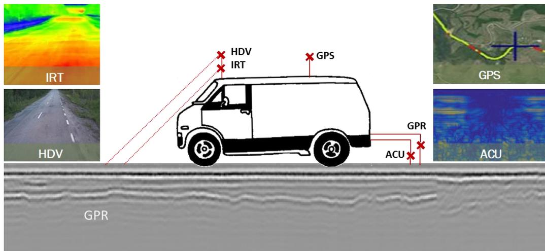
Figure 5. RPB HealTec system: NDT sensor data examples
