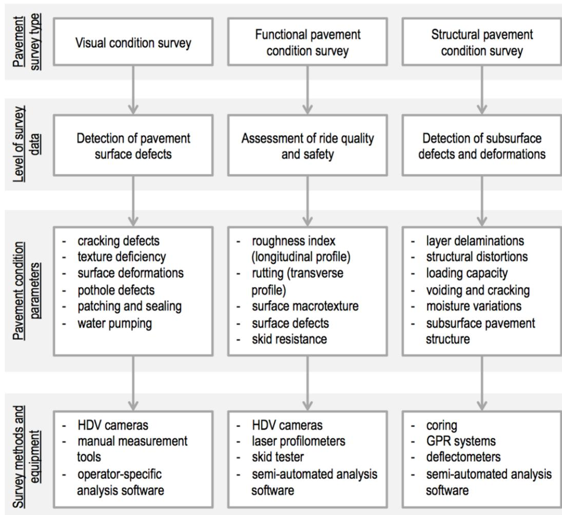
Figure 2. Road pavement survey types
