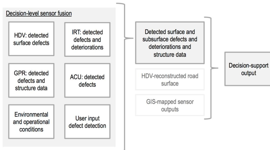
Figure 7. RPB HealTec system: NDT sensor fusion solution
