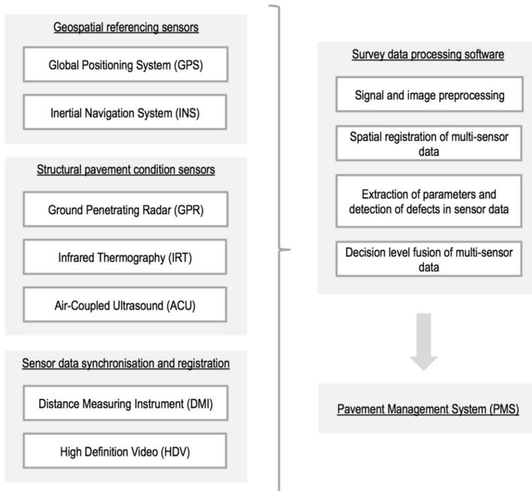
Figure 4. Design of the RPB HealTec system for pavement structural condition survey
