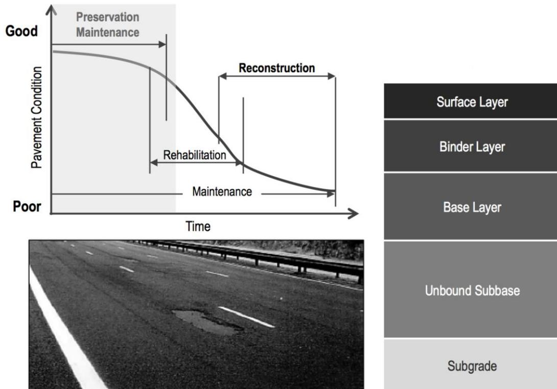
Figure 1. Flexible road pavement life cycle and general layer structure
