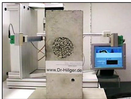
a. concrete sample with 10cm gravel nest and the USPC 4000 AirTech system
