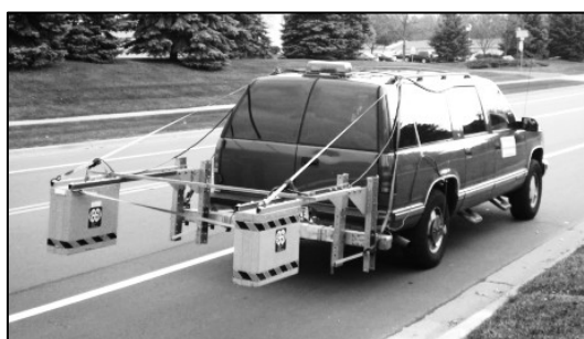
a. Air-coupled GPR system [2]
