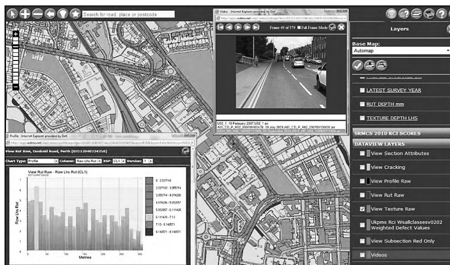
Figure 3.12 Example of pavement management software (WDM® pavement management system) [30]
