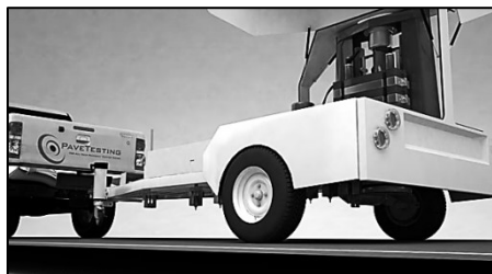
a. PaveTesting® FWD equipment [29]
