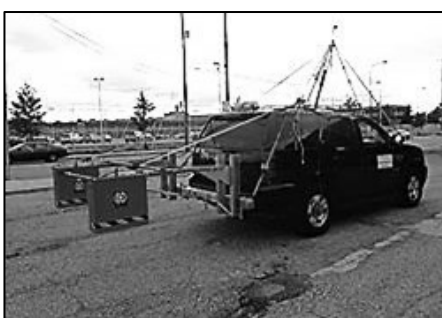
b. Infrasense, Inc. integrated GPR and IRT system [33]
