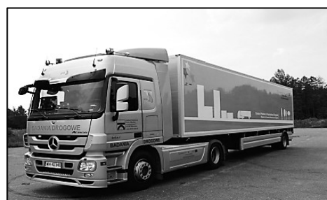
b. Traffic Speed Deflectometer [22]
