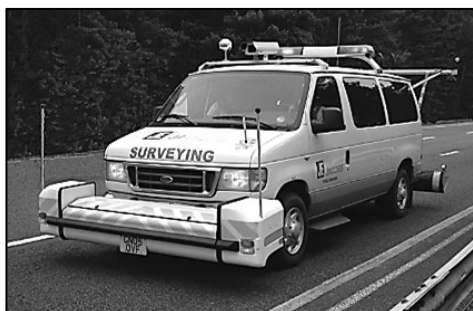
a. TRACS traffic speed pavement survey system [2]
