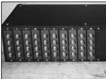
b. MIRA dry-coupled UT transducer array [36]
