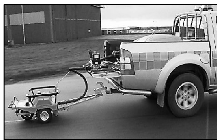
b. GripTester skid resistance measurement equipment [28]
