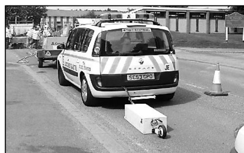
b. Ground-coupled GPR system [24]
