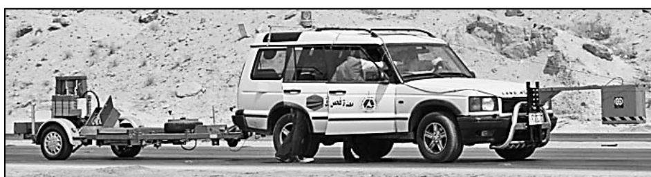
Figure 3.7 GSSI® Integrated GRP and FWD system [25]
