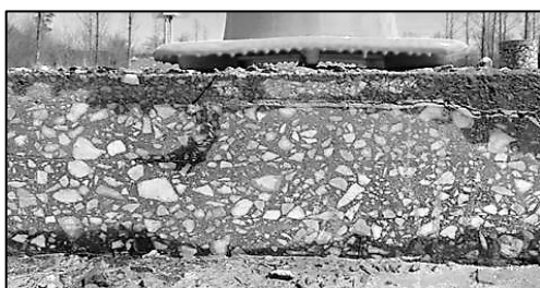
a. Debonding in HMA layers [23]
