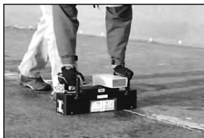
a. MIRA dry-coupled UT pulse echo equipment [36]
