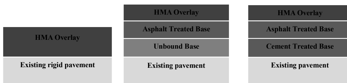
Figure 2.7 Common types of HMA surfaced composite pavements
