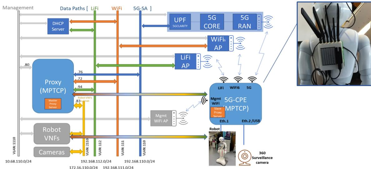
Fig. 2. MPTCP supported multi-connectivity testbed.
