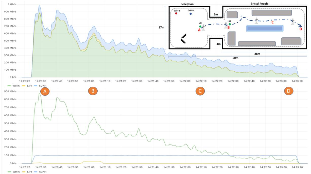
Fig. 4. Multi-RAT Uplink traffic for the cumulative and individual access networks.
