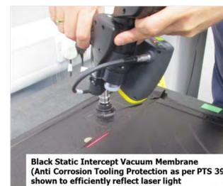
State-of-the-art laser line scanner provide accurate measurements of the thickness variability
