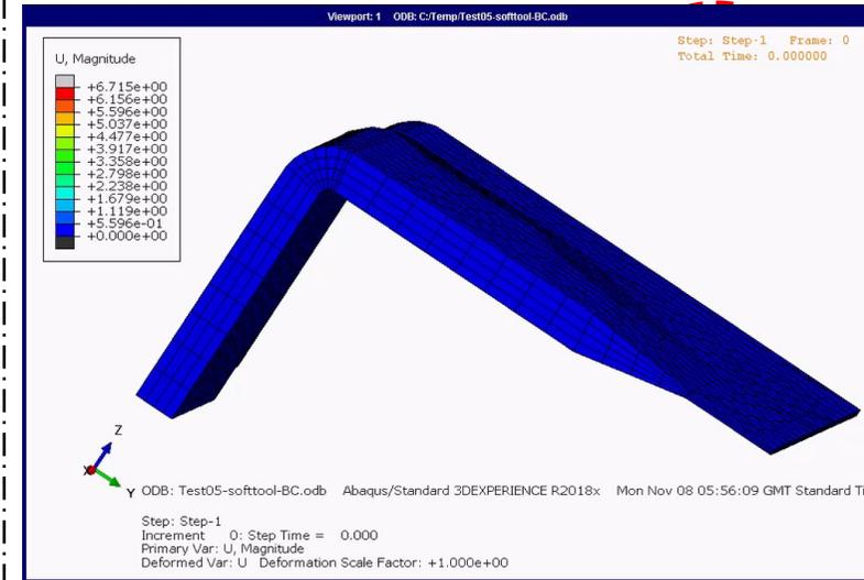
The output of the Virtual Autoclave with a representative result from vacuum bagging
