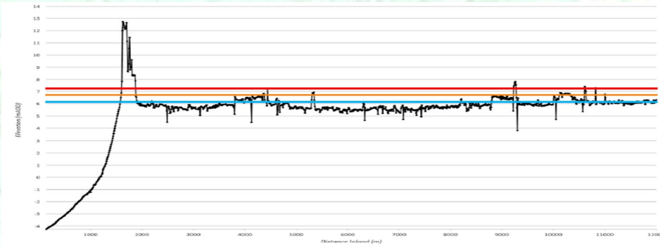
Figure 12: Elevation profile from Section B with the highest recorded astronomical tide (blue line) and the additional sea level rise projected in RCP2.6 (orange line) and RCP8.5 (red line)
