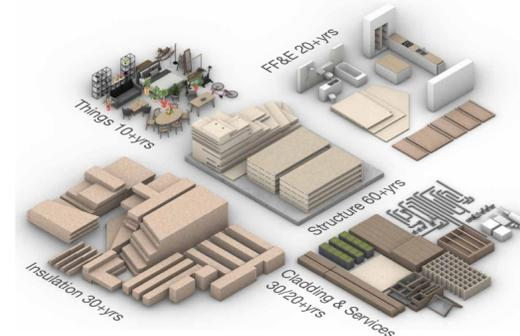
**Diagram 3: A kit-of-parts approach to manufacturing**
