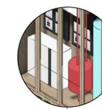
The brains of the house. Wireless technologies will enable flexibility. Hot water tank, a MVHR, electricity store and house computer will monitor and adjust the internal climate automatically.
