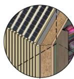
UK-grown C16+ graded Cross Laminated Timber with wood-fibre insulation and treated timber cladding manufactured in a local flying factory and assembled on site as a balloon frame.
