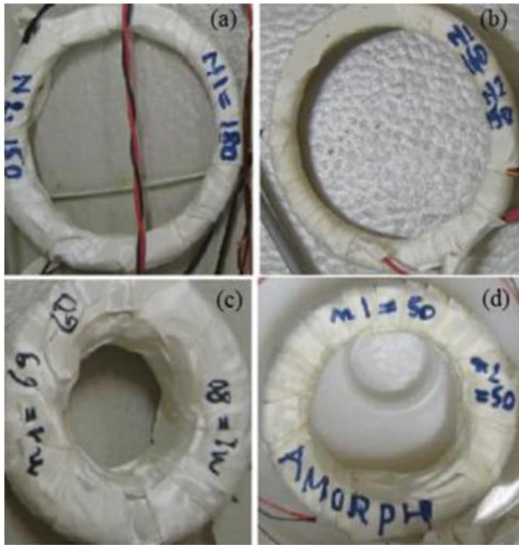
Fig. 1. Picture of soft magnetic ring core samples: (a) fully-processed, low loss non-oriented steel; (b) fully-processed, non-oriented steel with enhanced permeability; (c) grain-oriented steel; and (d) nano-crystalline alloy Finemet.
