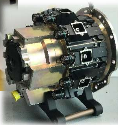
Motor/Generator with integrated Power Electronics
