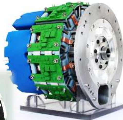
Motor/Generator with integrated Power Electronics
