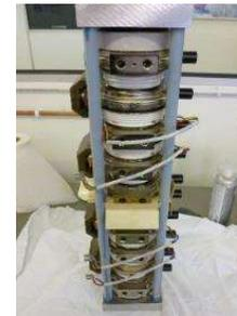
Class 92 Heatsink refurbishment (GTO and Diode)
