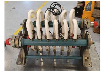
Class 91 Heatsink refurbishment (GTO and Diode)
