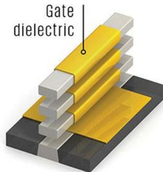
Atomic layer deposition builds a thin layer of dielectric on the silicon channels, including on the underside.
