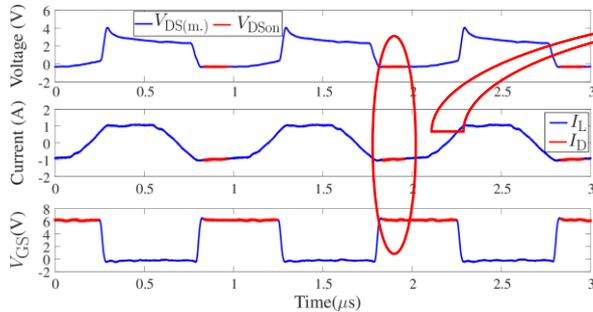
Measurement at the beginning of each duty cycle ( $f_{sw}=1\text{MHz}$ )
