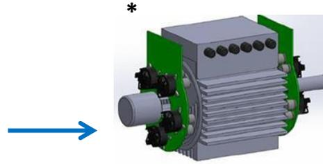
Integrated GaN power electronics circuit and systems
