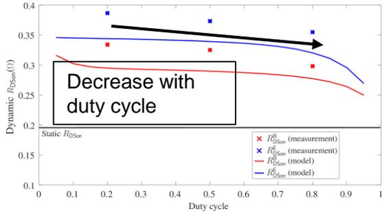
Different duty cycles ( $f_{sw}=100kHz$ )
