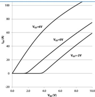
Figure 9 : Typical  $I_{SD}$  vs.  $V_{SD}$
