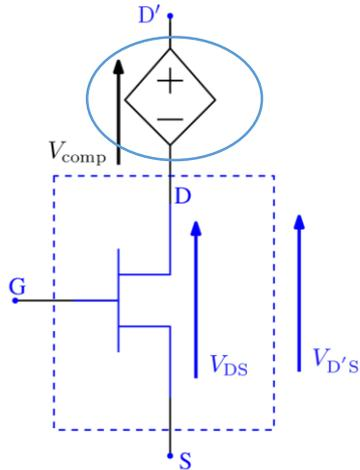
$$V_{DS}^{eff} = V_{D'S} = V_{DS} + V_{comp}$$
