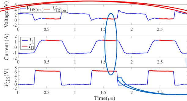
Measurement at the end of each duty cycle ( $f_{sw}=1\text{MHz}$ )
