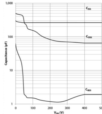
Figure 7: Typical  $C_{iss}, C_{oss}, C_{rss}$  vs.  $V_{DS}$
