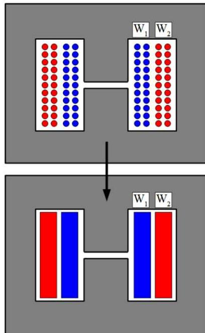
The SFD is based on an analytical loss expression in a single round conductor, assumed small compared to the skin-depth, subject to a uniform field.
