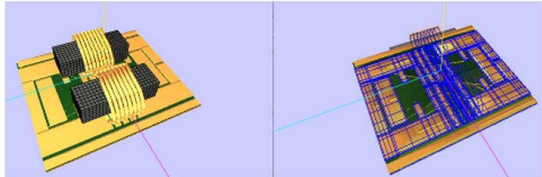
3D visualisation using ROM works for magnetic field and current density if matrix equation formulation modified
