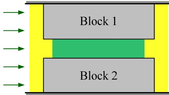
Flow network acts as fluid boundary condition for 3D coldplate model
