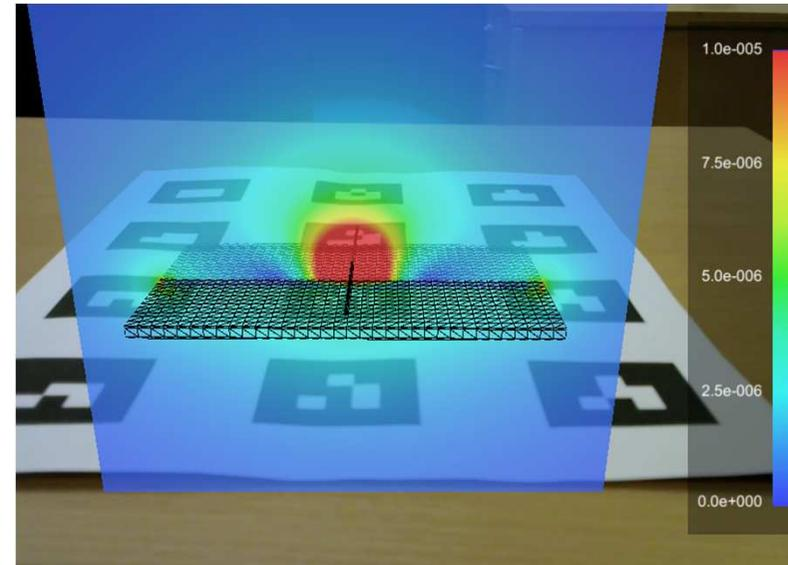
*Above – magnetic field, induced ground plane currents distort field at higher frequencies*
