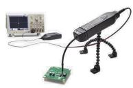
Optical isolation: 120 dB rejection of common mode
