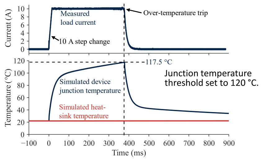
Demonstration of safe shutdown on highly overloaded GaN bridge-leg converter, operating at 10 A, 2 kW, and 500 kHz.
