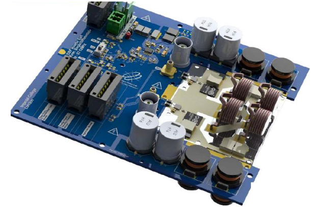
13MHz, 500W wireless power converter
