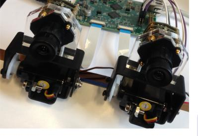
A two camera coupling motherboard allows a binocular pair to be configured. Two camera stacks with their own motion sensors and processing pipelines are coupled by the motherboard. Depth from vergence is implemented as a demonstrator; the motherboard has GPIO for pan/tilt motor control to be coupled with high ROI framerate visual tracking of the cameras.
