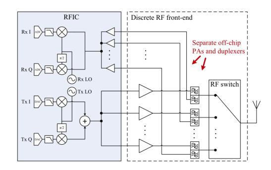
Acoustic filters (e.g. surface acoustic wave devices) are the only filters which can give the required performance, but these are difficult to tune, requiring multiple off-chip duplexers to support multiple bands. This increases cost, size and losses, and limits the number of bands which can be covered, restricting roaming.
