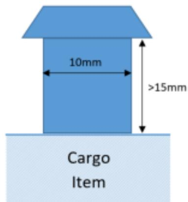
**Figure E-3: The Cylindrical Peg cargo interface**
