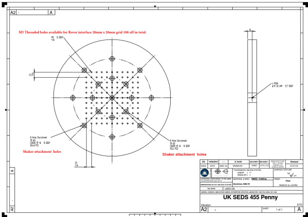
**Figure E-1: RAL Space Vibration interface plate**
