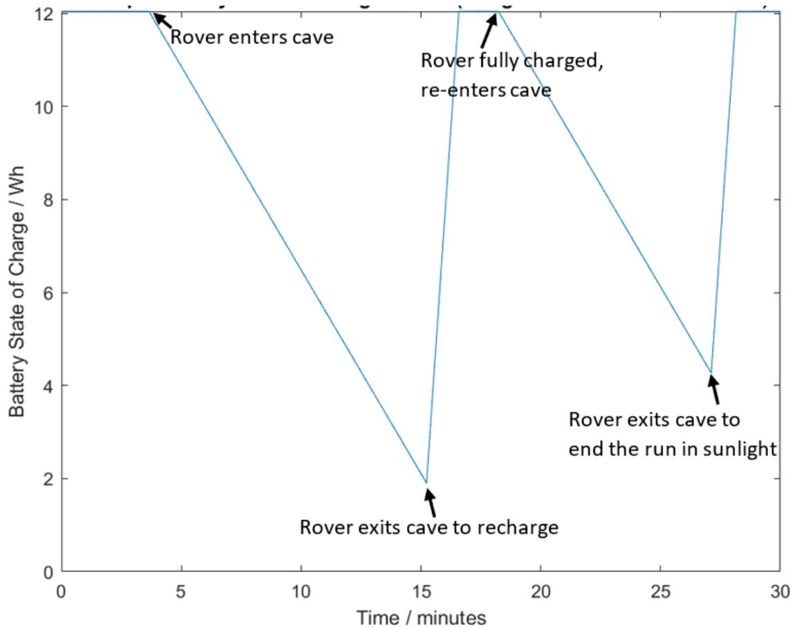
**Figure 2-1: Example Battery State of Charge Profile (3.5kg Rover with 5 Sparkwing Solar Panels)**
