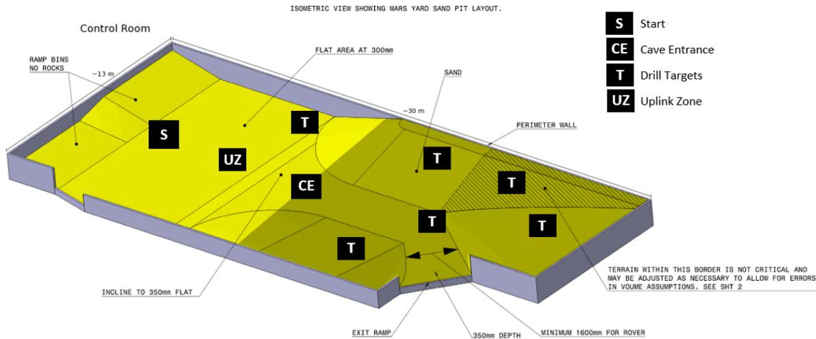
**Figure D-3: Airbus D&S Mars Yard - Topology Schematic - (Light and dark side of cave, with start, cave entrance and uplink zone shown. Drill target site locations demonstrated - these may change on the day)**
