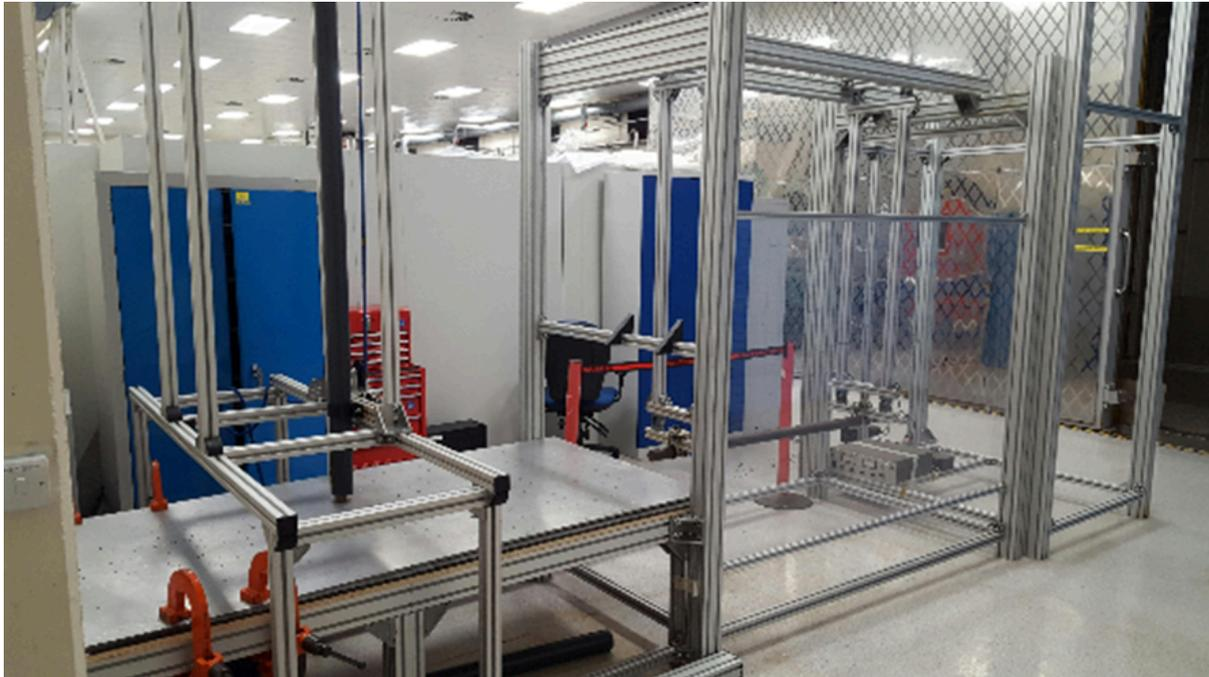
**Figure D-5: Shock Test Setup**
