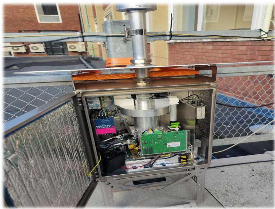
Swisens Poleno: Real time, speciated pollen concentration measurements. Using UV-LIF and holography camera to classification pollen species.
