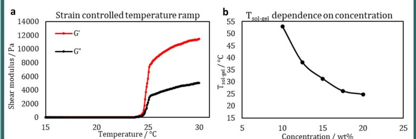
Figure 3- a) Example of a sol-gel transition of 20 wt% Poloxamer 407 exhibited by the extreme increase in storage and loss moduli.  $G'$  is the storage modulus (elastic component), and  $G''$  is the loss modulus (viscous component). In this case the sol-gel transition temperature is 24.5 °C. b) Sol-gel transition temperature of poloxamer 407 as a function of concentration. Each data point was found by plotting a strain controlled temperature ramp at varying concentrations.
