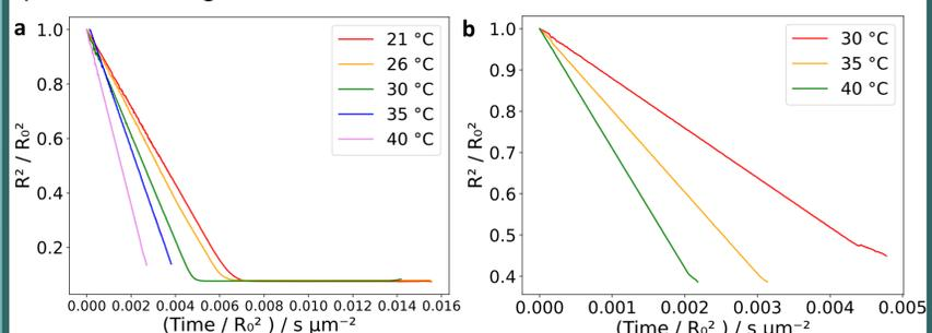
Figure 4—Normalised evaporation curves at different temperatures measured using the CK-EDB. a) 2.5 wt% Poloxamer 407 b) 0.2 wt% pNIPAM
