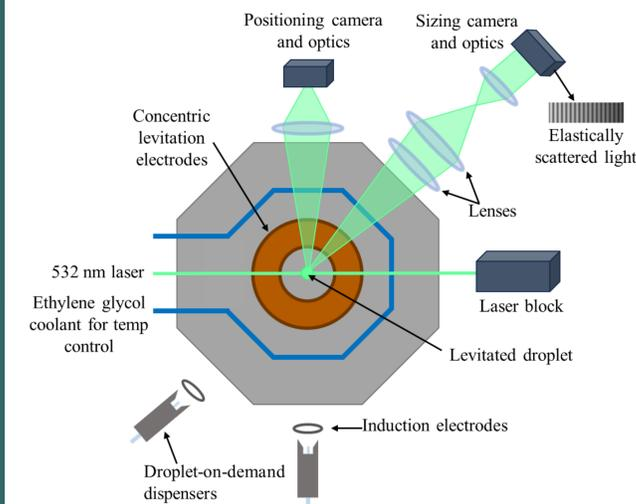
Figure 2—A schematic representation of a CK-EDB from a view looking down into the instrument.
