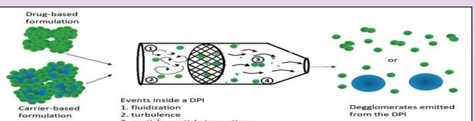
Figure 3. Schematic of DPI dispersion mechanism.<sup>12</sup>
