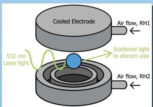
The EDB uses a combination of AC and DC electric fields to levitate a single charged droplet in place. Using scattered light from a laser, the size of the suspended droplet can be found.
