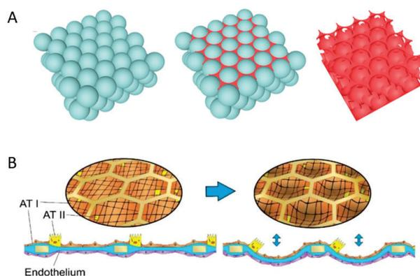
**Figure 3:** Second generation membrane designs for lung-on-chips. A) Reverse opal structure published by Huang *et al* <sup>37</sup> B) Zamprogano *et al* gold hexagonal mesh with collagen:elastin membrane.<sup>29</sup>
