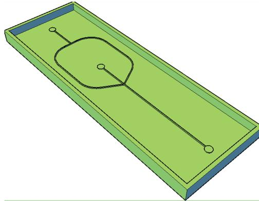
Figure 2: Master Mould for PLGA Synthesis
