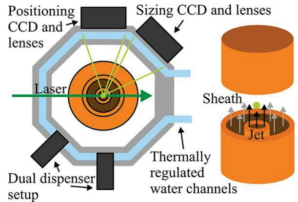
Figure 4: Experimental set up of CK-EDB [4]
