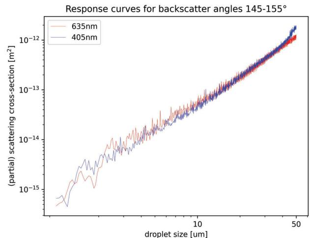
**Backscattered light response curve** – backscattered cross-section against droplet size, collected by an optic offset from the incident beam (0°) between 145 and 155° polar angles in red and blue wavelengths; non-monotonicity presents an uncertainty in the mapping of roughly ±2.5μm.
