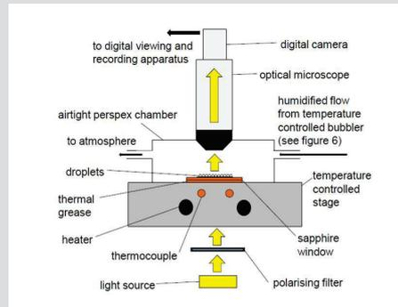
Figure 4. Schematic of the RH controlled chamber
