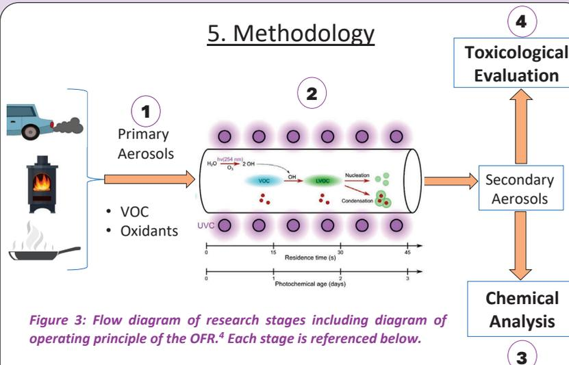
Figure 3: Flow diagram of research stages including diagram of operating principle of the OFR.<sup>4</sup> Each stage is referenced below.
