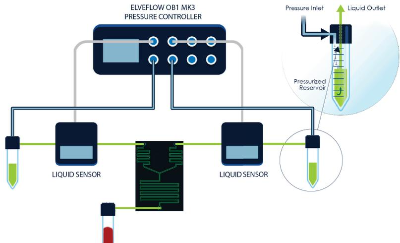
Figure 3: Microfluidic PLGA Synthesis Setup
