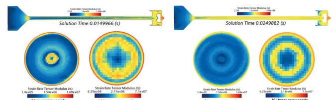
Fig.7. Strain rate of low-viscosity – water during atomisation
