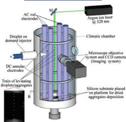
Figure 2 by Archer, Kolwas et al. 2019[1] illustrating the components of a quadrupole electrodynamic balance.
