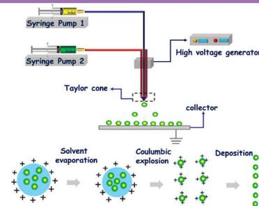
Fig 2. Schematic of electrospray drying
