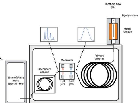
Figure 1: Diagram of the basic composition of a 2-dimensional Pyrolysis Gas chromatography instrument showing details of the modulator set-up and the effect of 2-dimensional separation. (created with Biorender)
