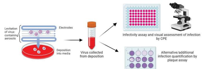
Figure 2: Workflow for determination of infection from levitation using CELEBS instrument.
