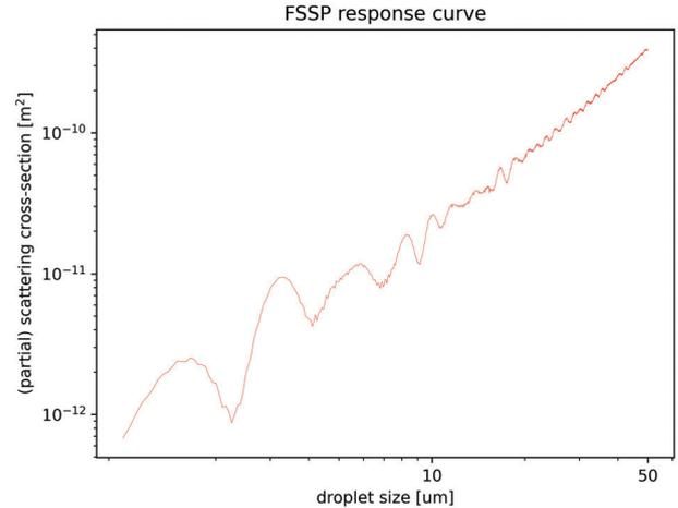
**Forward Scattering Spectrometer Probe (FSSP) response curve** – The FSSP collects forward scattered light from a 632.8nm red laser between 4.6 and 12.8° polar angles using an annular photodetector and has been widely used in cloud droplet research; the instrument response curve used to measure droplet size is replicated by the model [3], (the model is implemented in Python and uses the Python module *scattnlay* to calculate scattering amplitudes [4]).
