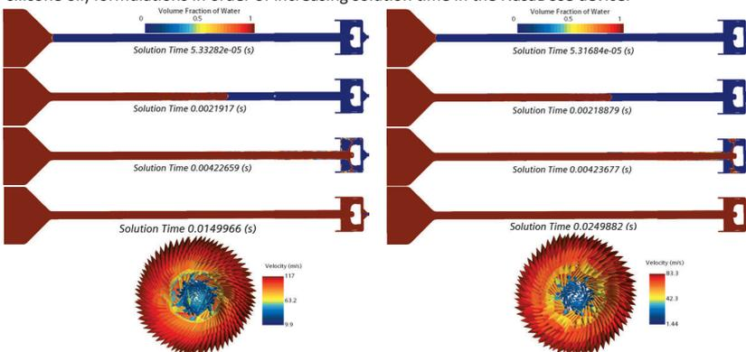
Fig.4. Fluid flow and nozzle Vector field for low-viscosity – water
