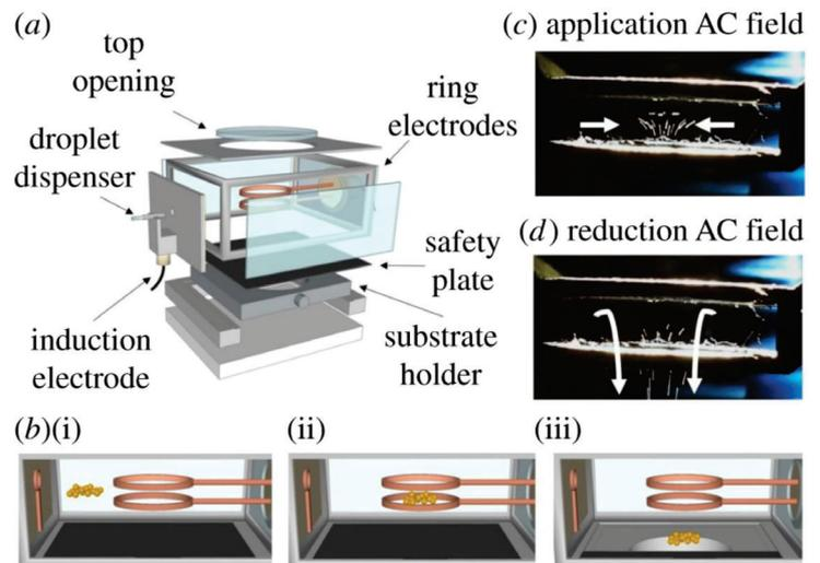
Figure 2. Schematic of the typical CELEBS setup and operating stages (a, b), images showing the levitation (c) and deposition (d) of a bioaerosol<sup>6</sup>.
