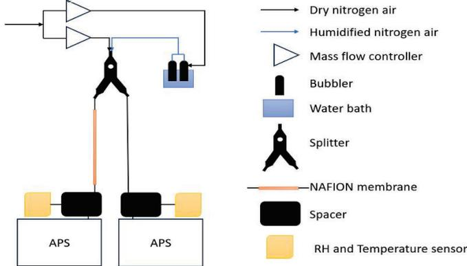
Figure 3: Experimental set up of TAPS [3]
