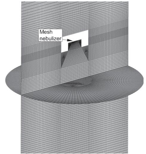
Figure 4: Hexahedral mesh of a spray dryer [4]
