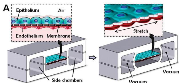
**Figure 2:** Huh *et al* First organ-on-chip, Emulate still use this design commercially. First generation design as the membrane only considers a single alveolar membrane as an extended structure.
