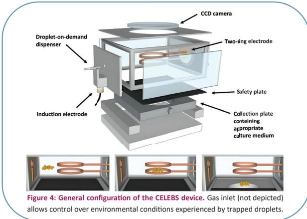
Figure 4: General configuration of the CELEBS device. Gas inlet (not depicted) allows control over environmental conditions experienced by trapped droplets.
