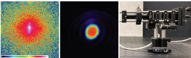
**(L) Backscatter Cloud Probe (BCP) beam profile** – The BCP is an existing backscatter instrument, but is limited for quantitative measurement [1]; variation of beam intensity within the sample area is one source of uncertainty.
