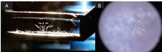
Figure 5: CELEBS generated droplets levitated in electromagnetic field. A) Side view of a population of droplets levitating in the CELEBS device. B) Overhead view of five droplets levitating in CELEBS device
