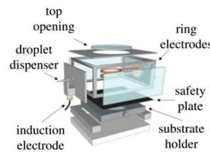
Figure 3 Schematic diagram of main components of the CELEBS apparatus<sup>[4]</sup>
