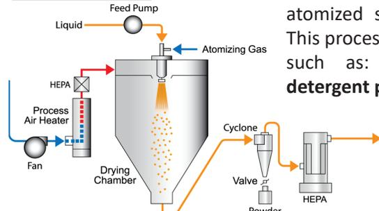
Figure 1: A schematic diagram of the spray dryer [1]
