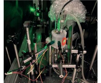
Figure 6. The concentric cylindrical electrodynamic balance
