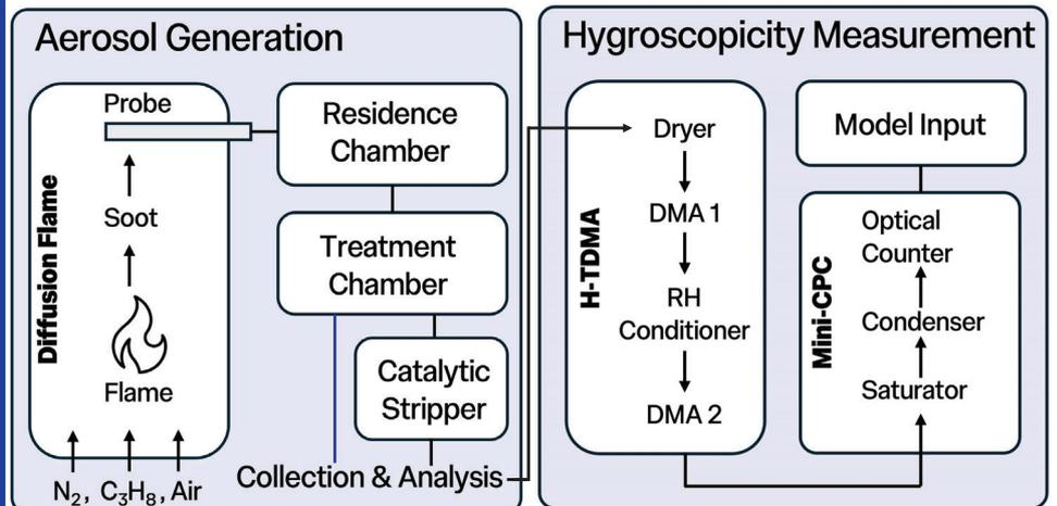
**Fig 4.** Schematic of proposed experimental set-up to parameterise hygroscopicity
