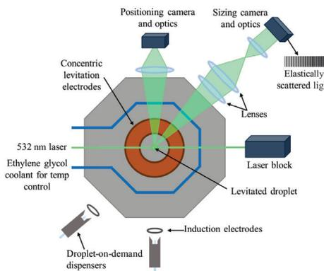
Figure 2—A schematic representation of a CK-EDB from a view looking down into the instrument.
