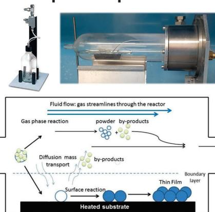
Figures 2, 3 and 4: A TSI 3076 aerosol generator, and schematics of an AACVD reaction chamber. [3][4]
