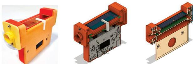
Figure 1: A portable electrostatic precipitator aerosol sampler in development at The University of Hertfordshire
