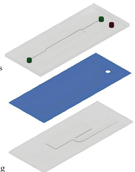
Figure 4: OOC Chip Design with Pneumatic Actuation
