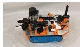
Fig. 1. In April 2022, the robot Lyra completed a survey of a 140m long radioactive ventilation duct below a disused laboratory at the Dounreay nuclear complex<sup>6</sup>.
