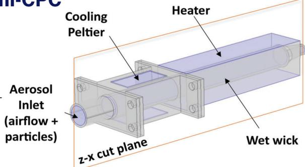
**Fig 5.** Schematic of mini-CPC device taken from Balendra *et al.* [6]
