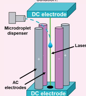
Figure 4: Schematic of the LQ-EDB.
