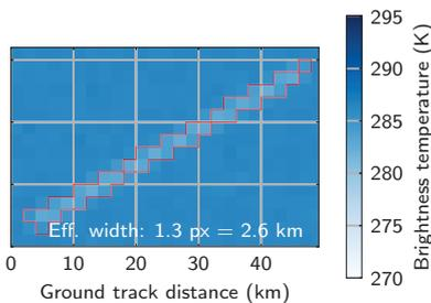
**Fig. 1** A 2 km resolution simulated contrail image
