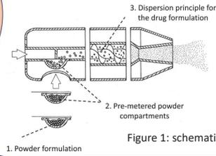
Figure 1: schematic of a DPI
