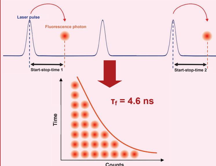
Figure 1: A pictorial representation of TCSPC and the histogram produced of the fluorescence decay from which a time constant is established.<sup>4</sup>
