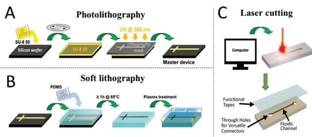
**Figure 4:** Fabrication methods of Organ-on-chips.
