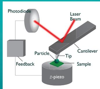
Figure 2 (Adapted from [4]): Schematic of a colloidal probe atomic force microscope.
