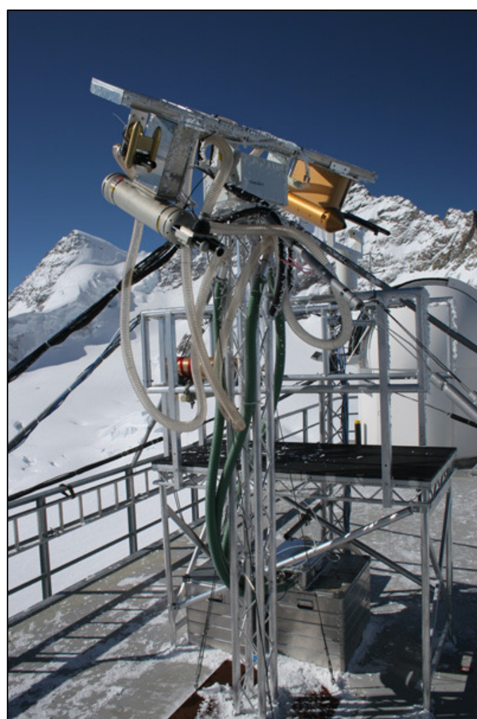
Sphinx Observatory, Switzerland (3,571 m) – Costly aircraft cloud spectrometers require scaffolding and modification for ground-based use [6].
