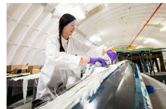
Figure 5. Example of manufacture of a thermoplastic composite turbine blade 5
