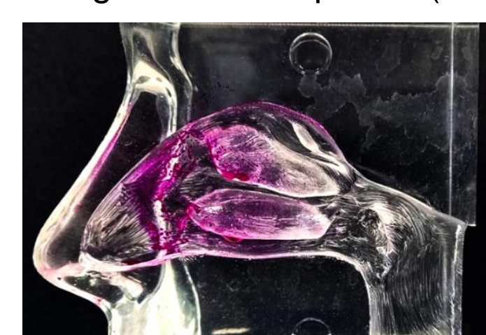
Fig. 10. Illustrates a deposition profile examine using dye-based imaging on a nasal cast (Upperton).
