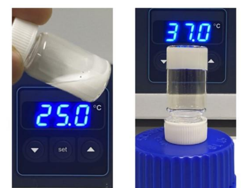
Fig. 4. Illustrates the effect of temperature on viscosity of a thermoresponsive gel.
