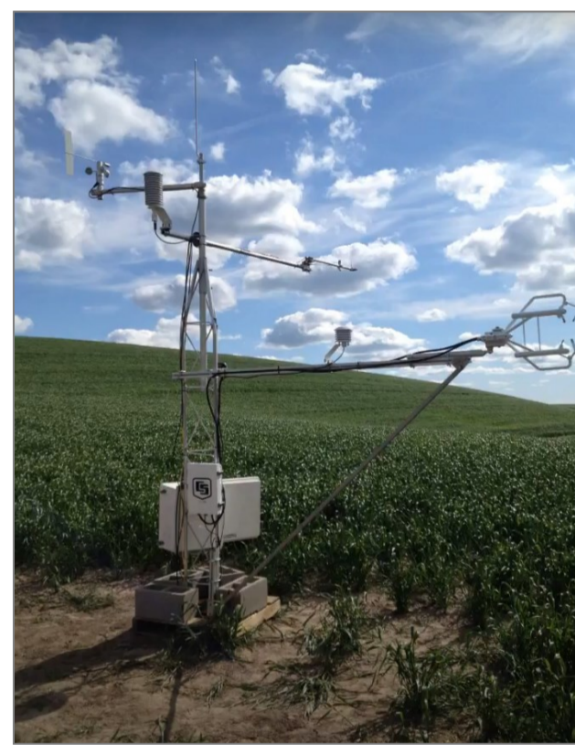
Fig. Eddy correlation system for gas measurement
