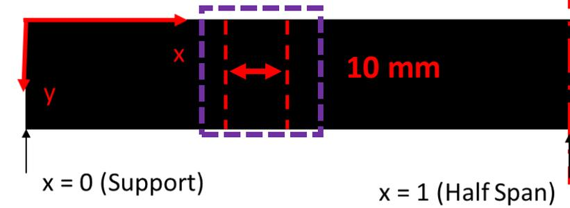
10mm debonded specimen loaded at -550N mean load with  $\pm 450$ N amplitude
