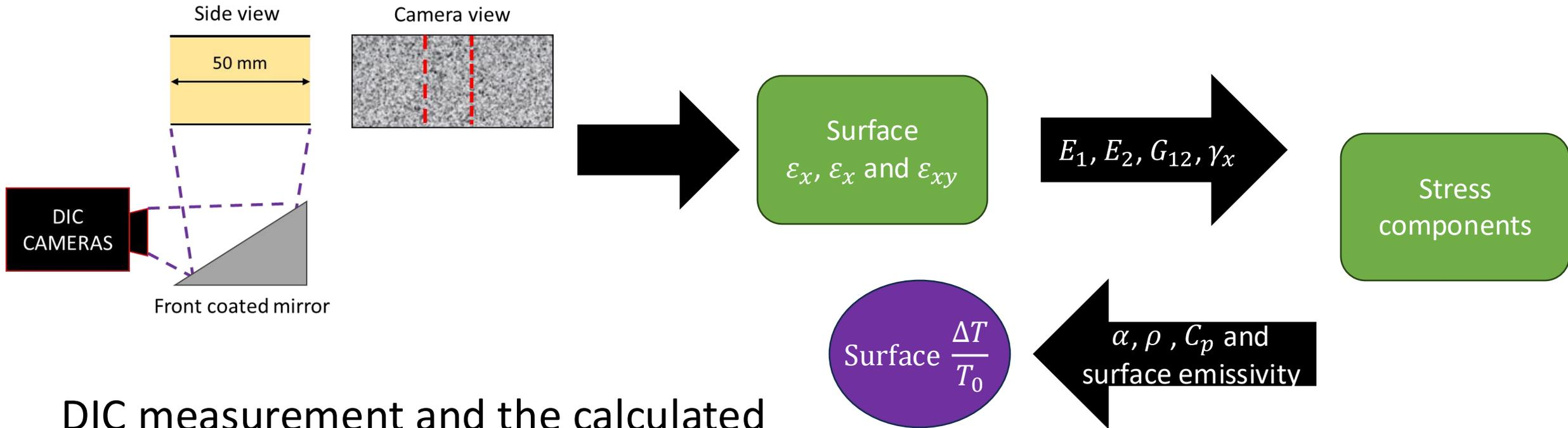
DIC measurement and the calculated surface  $\frac{\Delta T}{T_0}$  are independent of the heat diffusion effect
