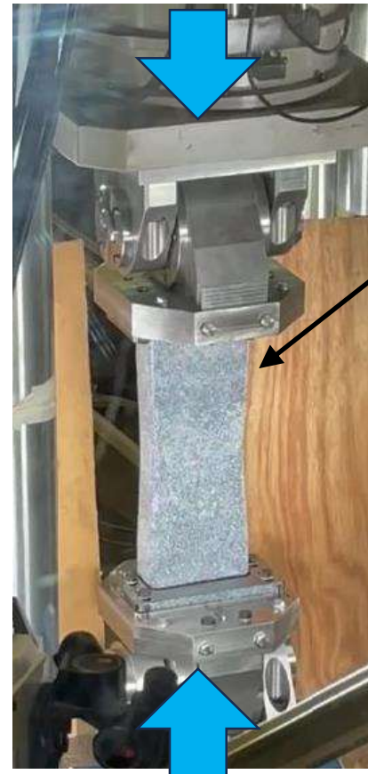
Test fixture design showing boundary conditions
