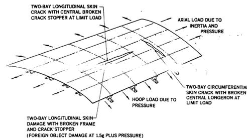
FIGURE 2. FUSELAGE DAMAGE TOLERANCE SIZES FOR STRUCTURAL DESIGN
