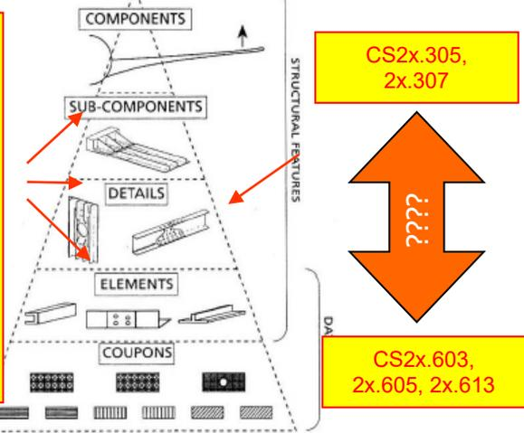
Figure 1 - Schematic diagram of building block tests for a fixed wing.
