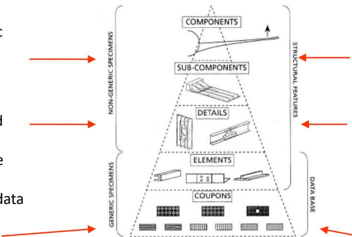
Figure 1 - Schematic diagram of building block tests for a fixed wing.
