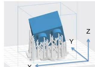
e.g. support structure on the build platform
