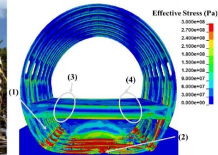
(b) Section drop test simulation result
