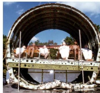
(a) Post-impact picture of section drop experiment
