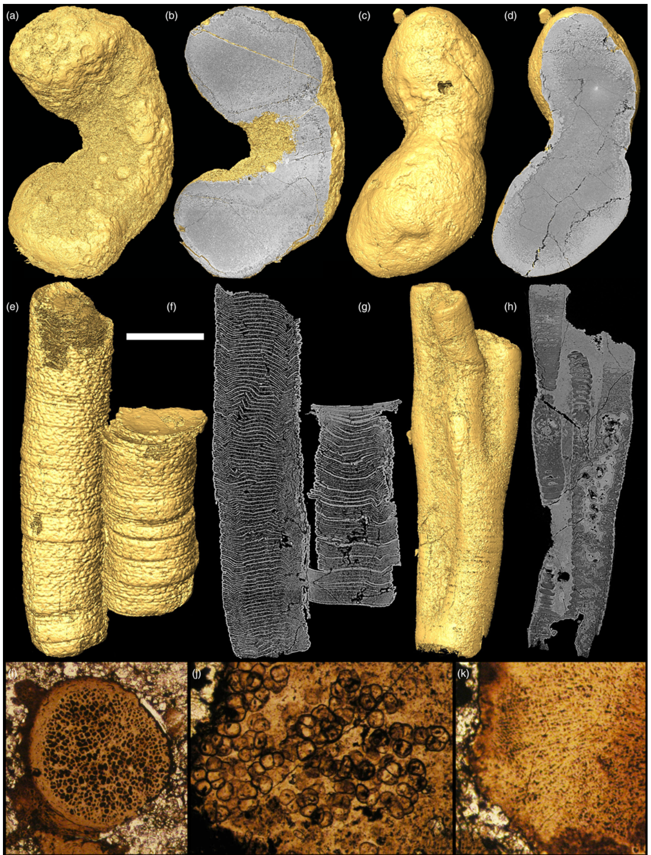
Fig. 3. Synchrotron radiation X-ray tomographic microscopy (SRXTM; a–h ) and light microscopy ( i–k ) images of Weng'an fossils. ( a, b ) a possible alga SMNH X 6459, comparable with Paramecia . ( c, d ) a peanut-shaped fossil SMNH X 6460. ( e, f ) Sinocyclocyclicus SMNH X 5322. ( g, h ) Ramitubus SMNH X 5326. ( i–k ) Light microscopy images of putative algae from Weng'an. Scale bar: ( a, b ) 270 \mu\text{m} , ( c, d ) 280 \mu\text{m} , ( e, f ) 180 \mu\text{m} , ( g, h ) 175 \mu\text{m} , ( i, j ) 140 \mu\text{m} , ( k ) 115 \mu\text{m} .
