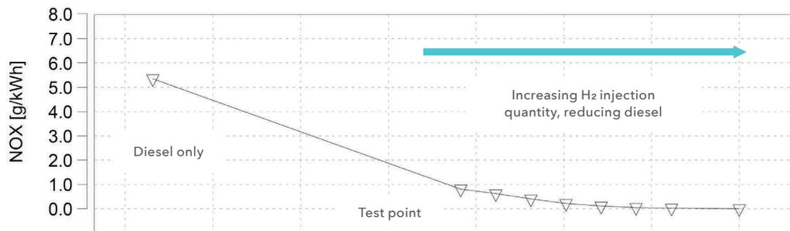
from hydrogen, with varying injection timing for the diesel pilot injection. The advanced injection reduces NOx to virtually zero by creating a multi point ignition behaviour similar to homogenous charge compression ignition engines.
