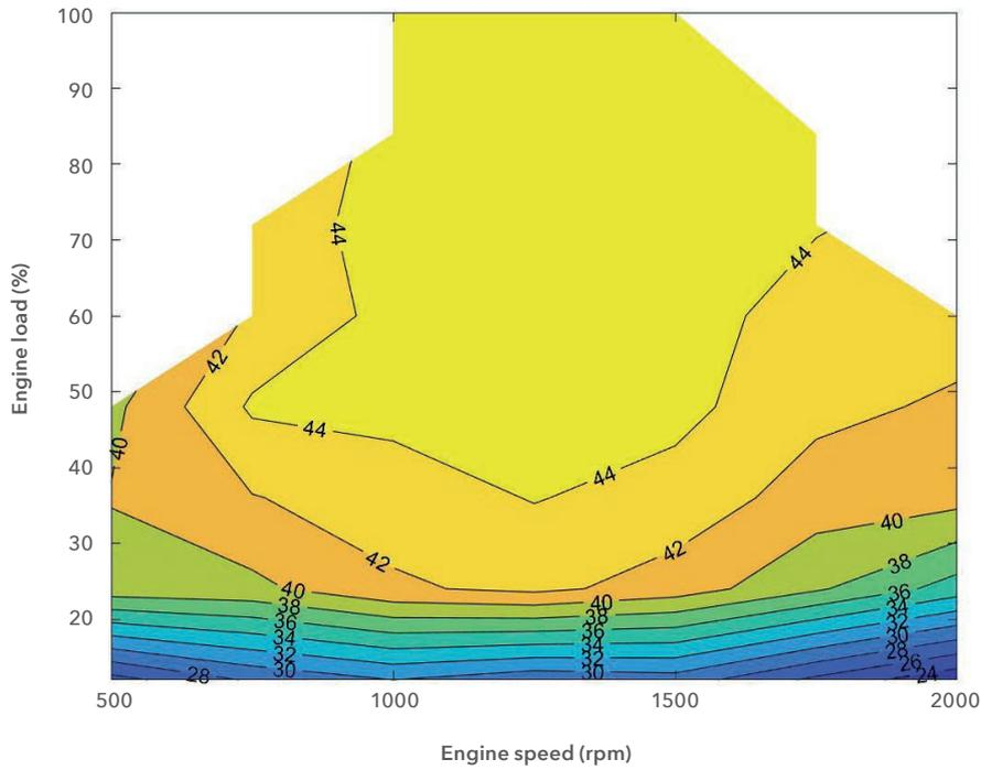
Figure 3: Brake thermal efficiency contour plot for a hydrogen engine
