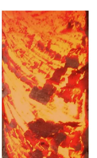
The benefit of twisting the billet is that the billet goes from a basic horizontal layered pattern, to amalgamating all the interior layers and warping the outer layers around the billet. It has a predictable outcome while the billet is still square/round, a twist up the billet, however when this is forged flat the twist gets compressed into itself. After thorough forging and grinding this reveals a crazy less predictable pattern.
